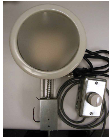
Figure 20. Fixture of 6" downlight with integrated driver and Triac dimmer
